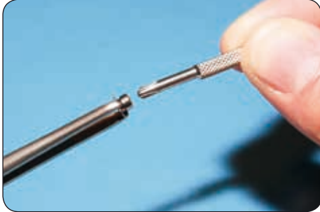
7: Adjustment of the retention with the activator.
