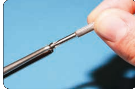
8: Each 1/4 rotation increases/decrease retention strength by approx. 200g.
